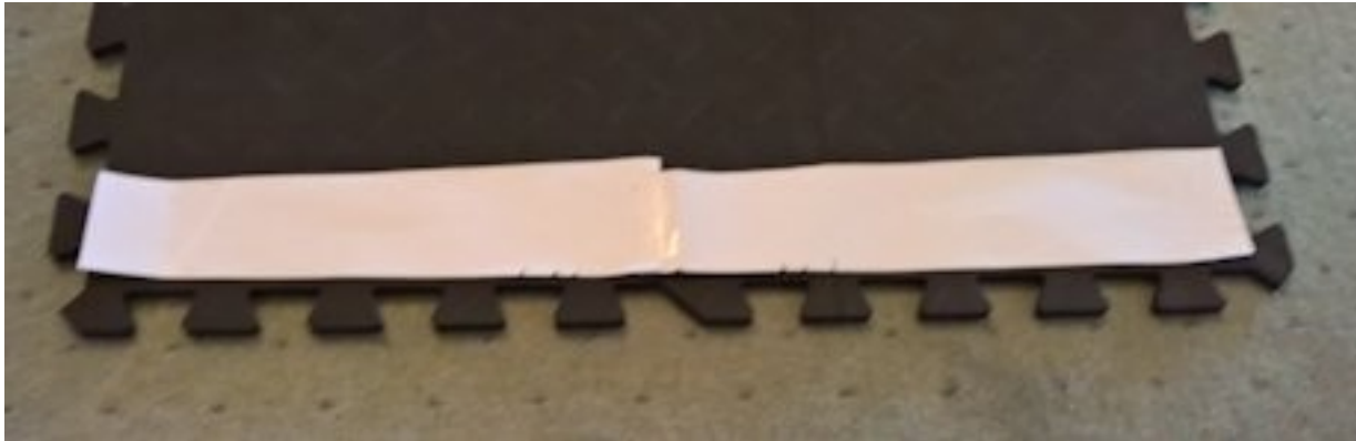
A paper strip used for easy marking of points along the edges of tiles.
